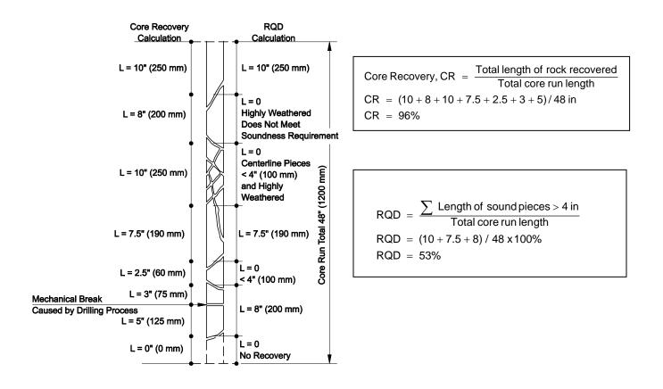
Figure 8.3-C — CALCULATION OF CORE RECOVERY AND RQD
